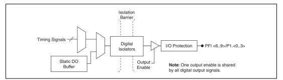
Figure 8-2. NI 6232/6233 PFI Output Circuitry
